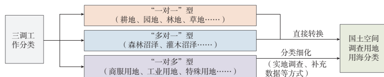
图4 三调分类与用地用海分类转换衔接关系图 Fig.4 The relationship between the survey data classification and the planning data classification
